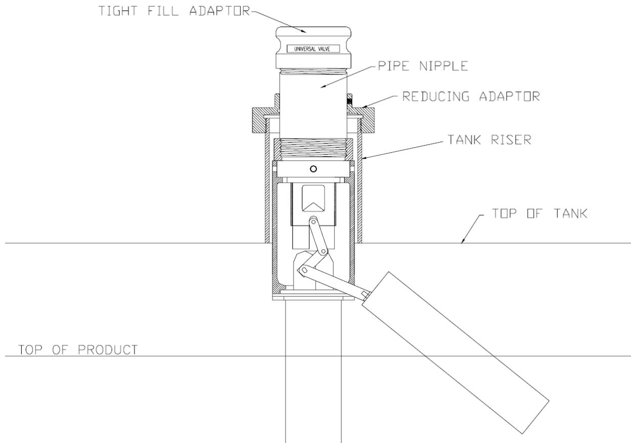
**Figure 2 Typical Fuel Storage Tank with Model 49**
