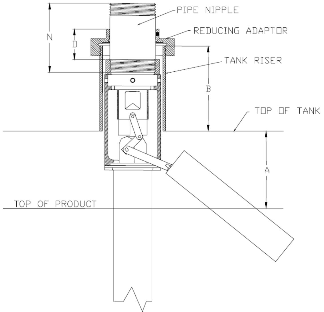
**Figure 1 – Model 49 Overfill Prevention Valve
