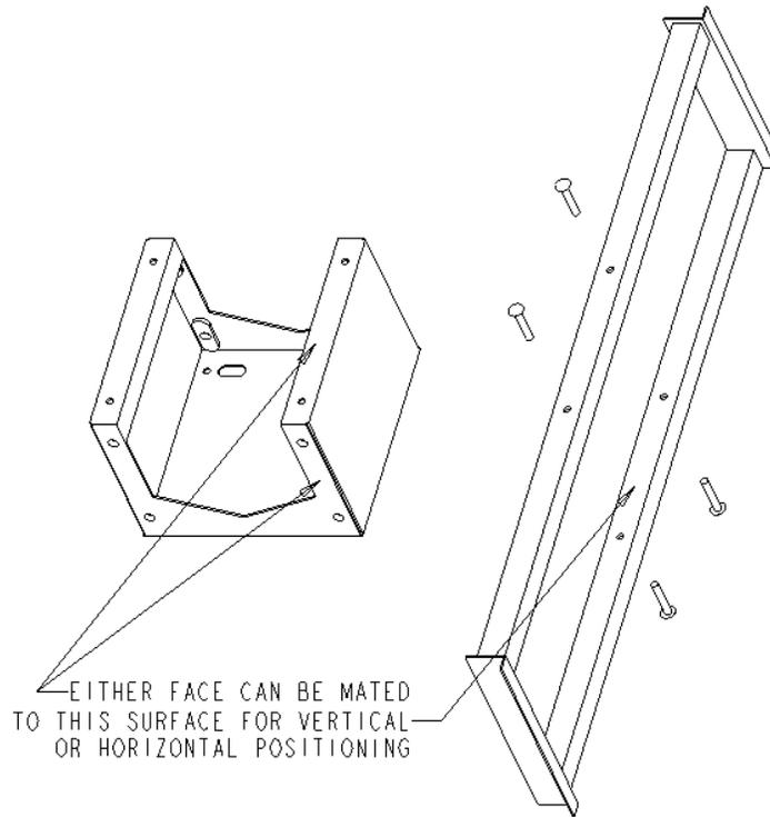
2. Place U-Clamp Box on the frame that is already mounted on back of BumperBoard™, aligning bolt holes. U-Clamp Box may be oriented in any position for mounting in horizontal or vertical position. (See Fig. Above)
